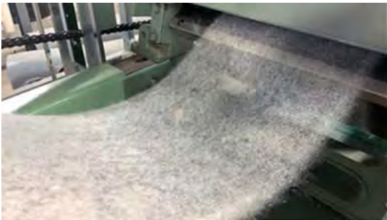
Cotton web containing the copper oxide nanoflowers produced in the Cotton Textile Mill pilot plant using a mini-carding system. It can be used as is, or further processed to create durable nonwoven fabrics. (Photo courtesy of Matthew Hillyer)
